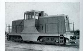
The 65-ton diesel-electric has a driving motor on each axle for high hauling capacity.
