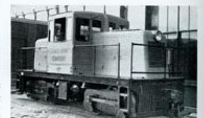
Steeple cab and low hoods on the 45-tonner afford excellent visibility in all directions.
