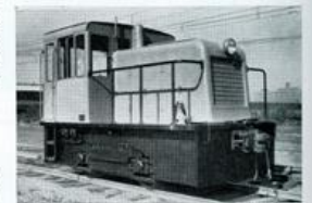
This 25-ton size can be furnished in gages from 36 inches to standard.
