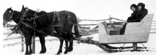
A "Shaganappi Cutter" in the Beaverlodge area of Alberta. n.d. Glenbow Museum Archives NA-649-19. It was a home-made box built over the front bob of a sleigh.
